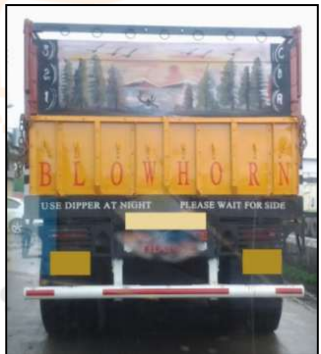
Fig. 2 Rear Simple Underride Protection in truck
