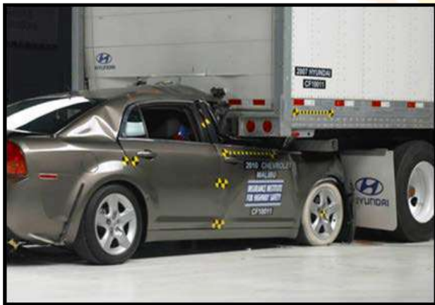
Fig. 4 A test for the anti-collision equipment's [3]
