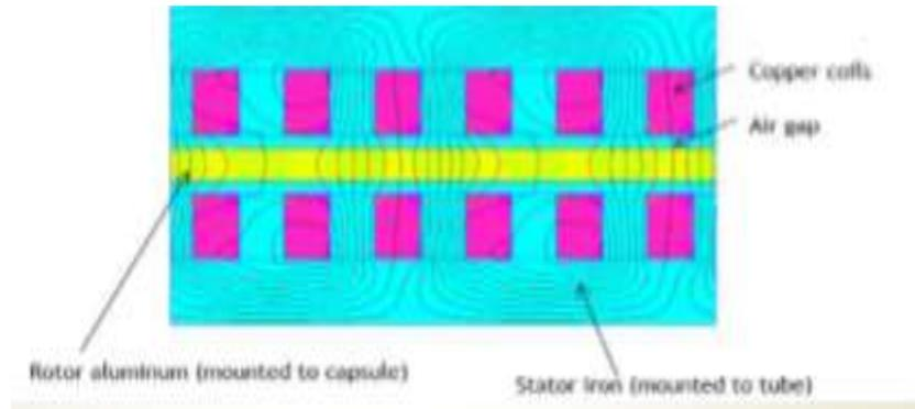
The rotor of the linear accelerators is very simple – an aluminum blade 49 ft (15 m) long, 1.5 ft (0.45 m) tall, and 2 in. (50 mm) thick . Current flows mainly in the outer 0.4 in. (10 mm) of this blade, allowing it to be hollow to decrease weight and cost. The gap between the rotor and the stator is 0.8 in. (20 mm) on each side. □ A combination of the capsule control system and electromagnetic centering forces allows the capsule to safely enter, stay within, and exit such a precise gap.
