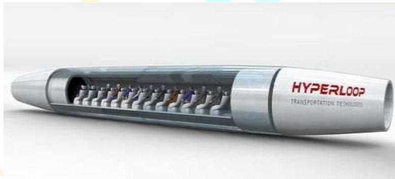
Sealed capsules carrying 28 passengers each that travel along the interior of the tube □ A larger system has also been sized that allows transport of 3 full size automobiles with passengers to travel in the capsule. □ The capsules are supported via air bearings that operate using a compressed air reservoir and aerodynamic lift.
