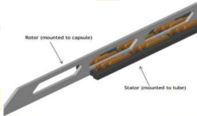
Linear accelerations are constructed along the length of the tube at various locations to accelerate the capsule. Stators are located on the capsules via the linear acceleration.
