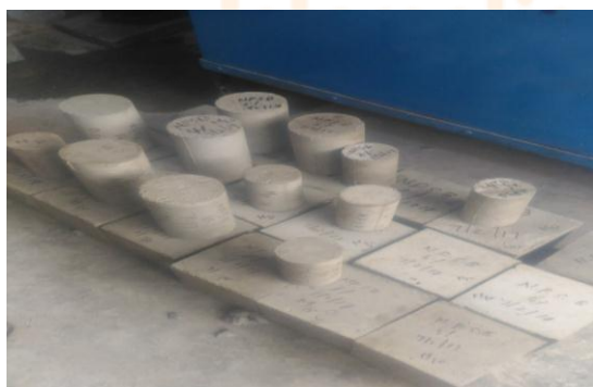
Fig 5: cube & cylinder for compressive, split tensile test
