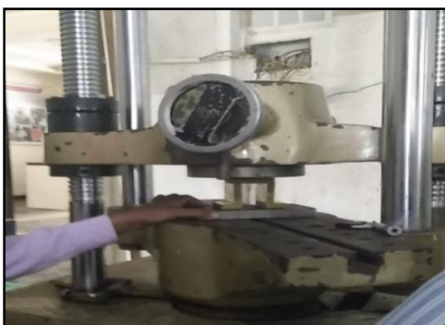
Fig.21.Compression loading of a GFRP bracket
