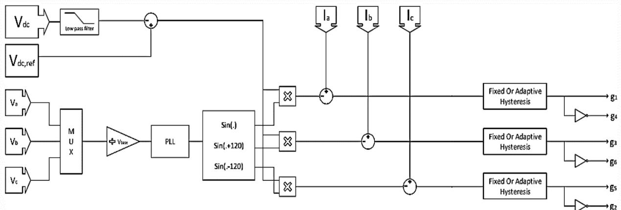
Figure III-1 Block diagram of the grid interface VSC controller
