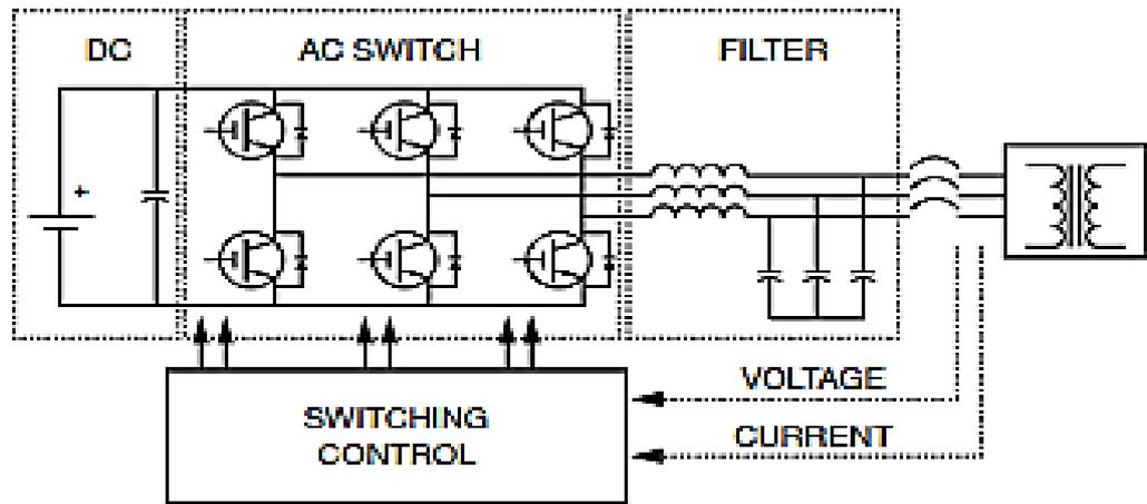
Figure II-1 Simplified Schematic Diagram Of A Modern Switching Inverter
