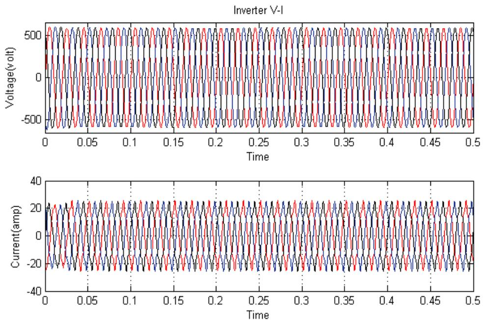
Figure V-7 inverter voltage current
