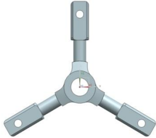
Fig: shows the 3D model of Helicopter rotor Hub (top view)
