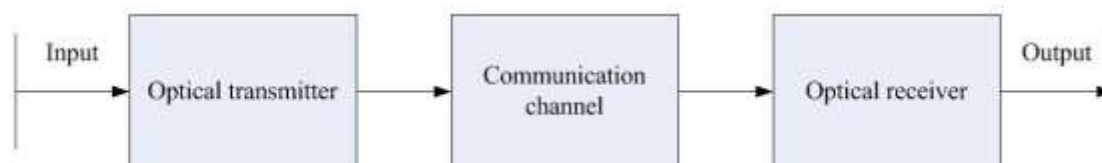
Figure 2 Block diagram of an optical communication system
