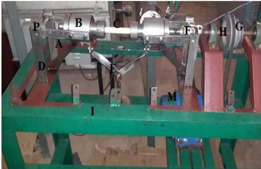
A- Horizontal Lever B- Bearing Housing C- Specimen D- Vertical Rest E- weight hanger F- Universal Joint G- Stepped Pulley H- Power Transmission Shaft I- Base M- Phase Motor ,P-Pivot
