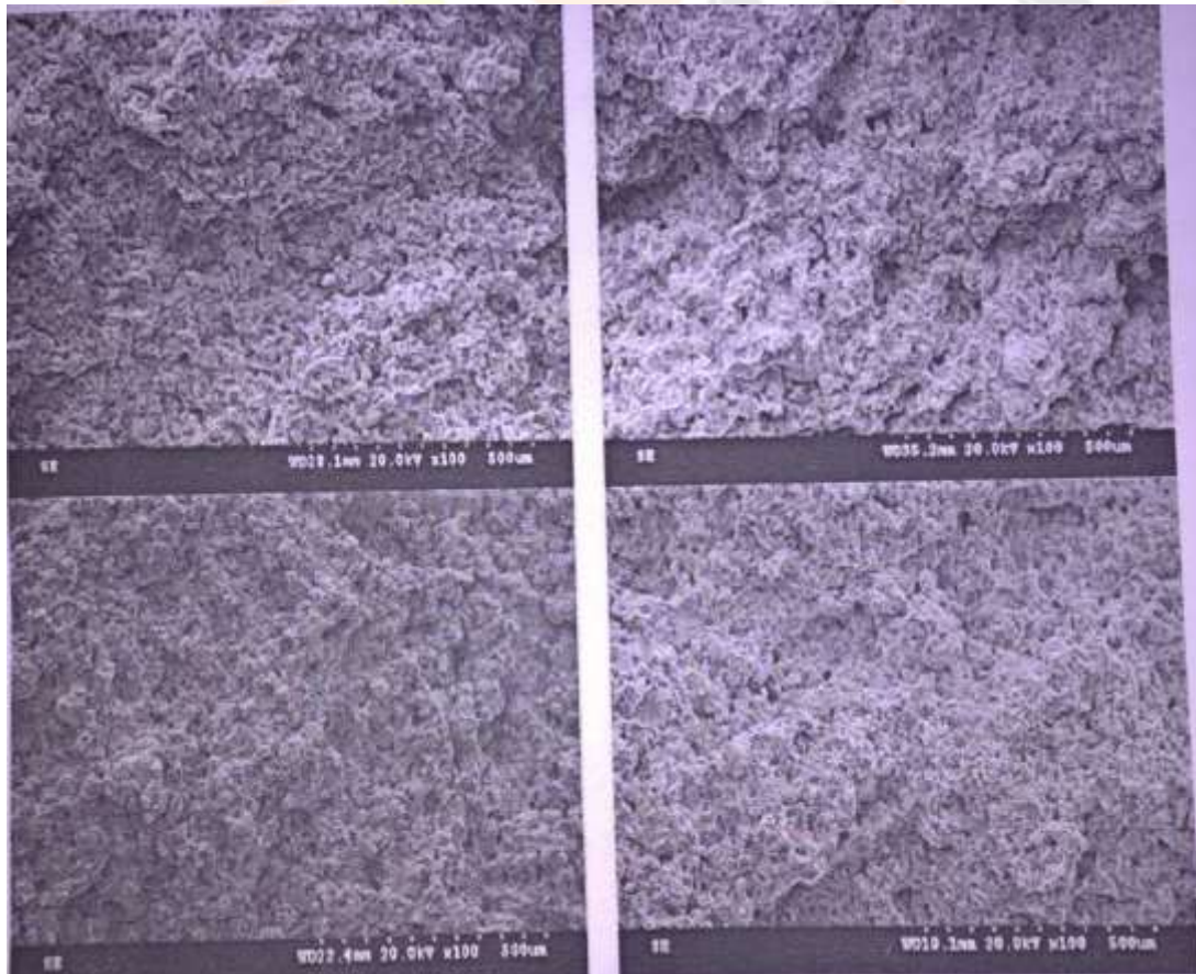
Figure 8. The fracture surfaces of PM steels in SEM analysis.
