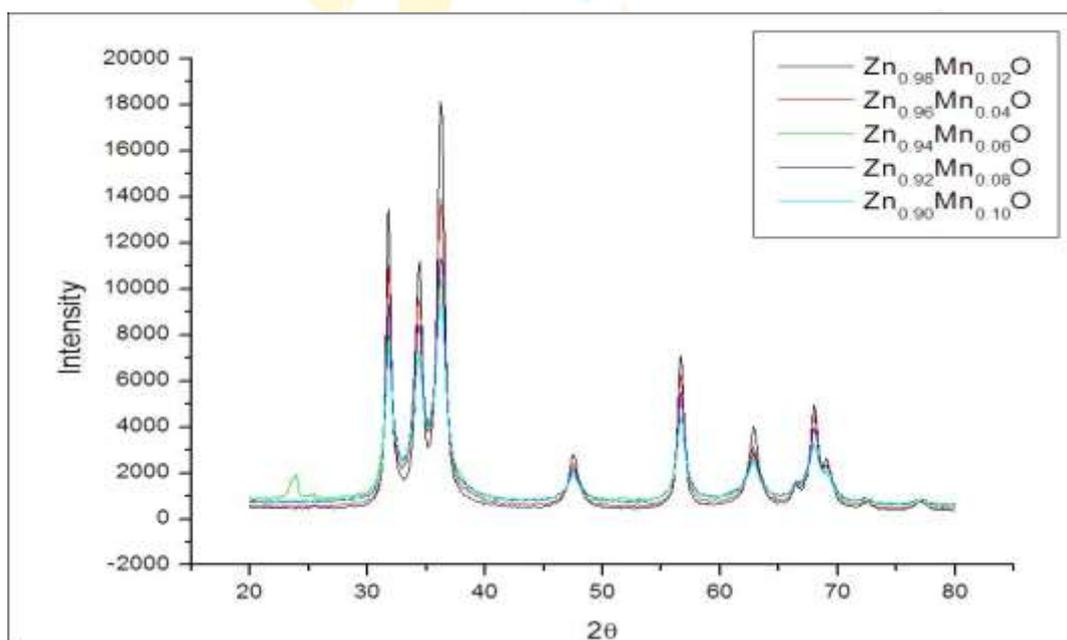
Figure:3 XRD pattern of 2% wt., 4% wt., 6% wt., 8% wt., 10% wt. Mn doped ZnO
