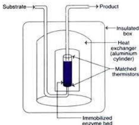
**Fig 6: Thermometric Biosensor**
