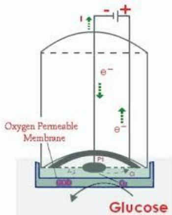
**Fig 2:** Glucose biosensor
