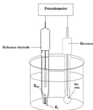
**Fig 3:** Potentiometric Biosensor.
