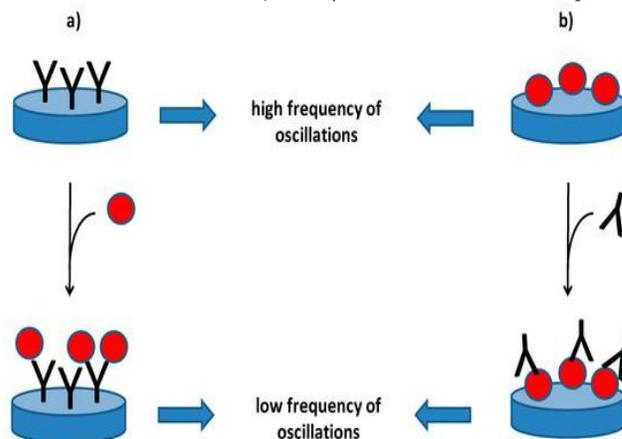
**Fig 5: Piezoelectric Biosensor**
