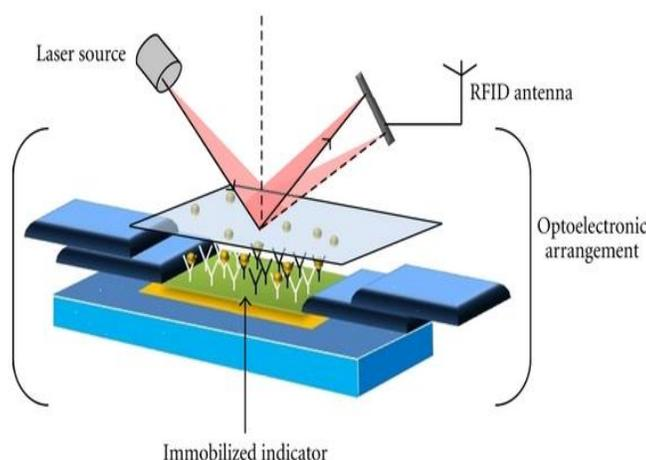
**Fig 7: Optical Biosensor**
