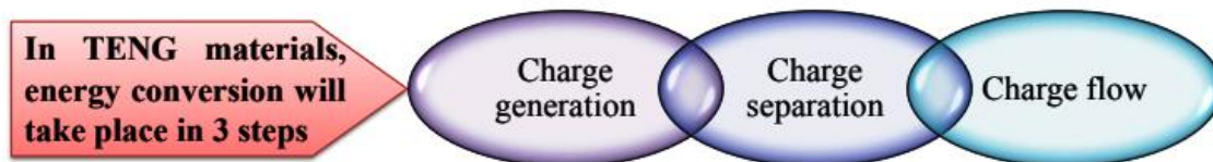
Fig2. Energy conversion in TENG material
