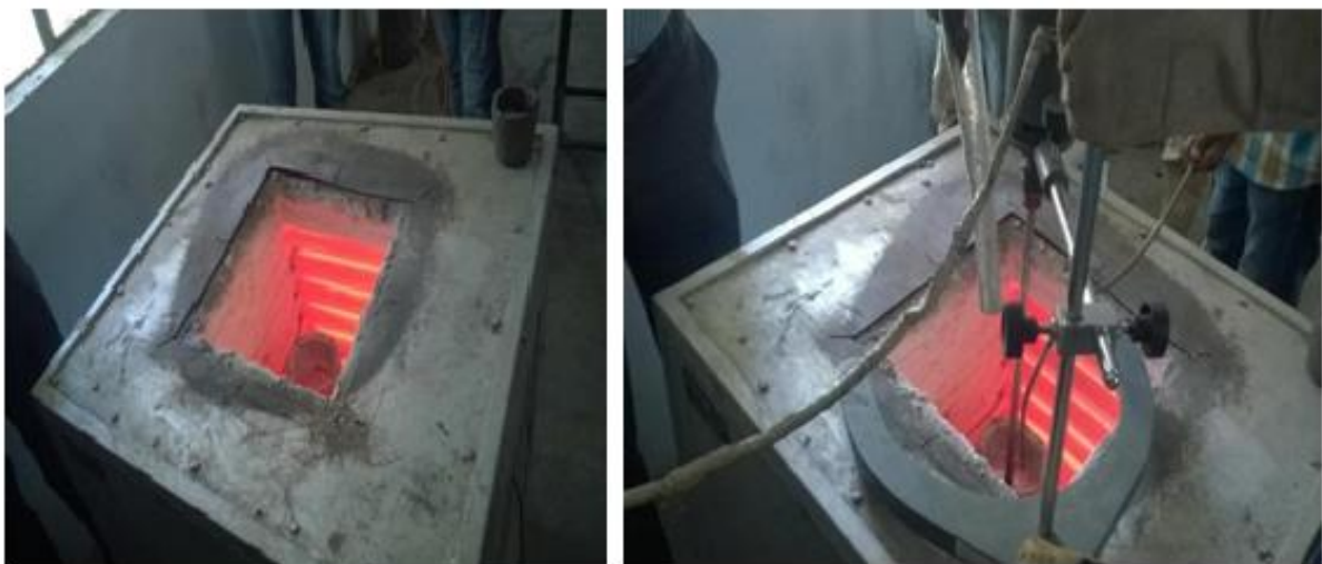
Figure.1 Electrical Arc Furnace with Stir Casting Method
