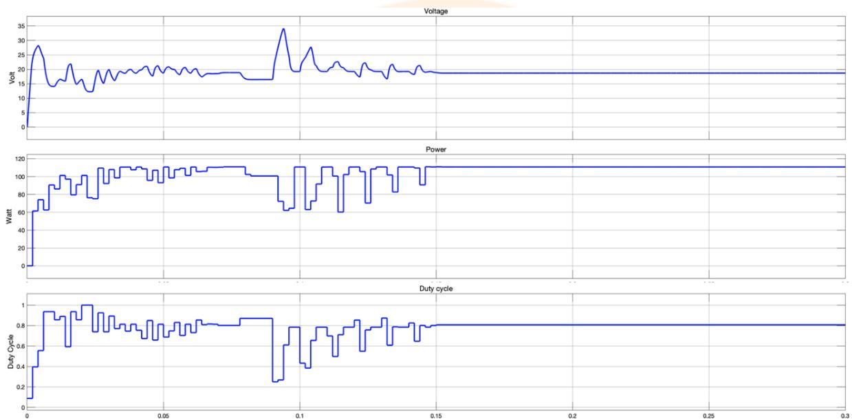
**Fig. 4 Performance of Proposed PSO MPPT under Variable/partial Shaded condition**
