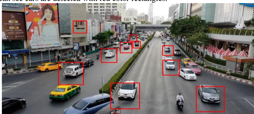
Fig: Detection and tracking of cars from input video stream
