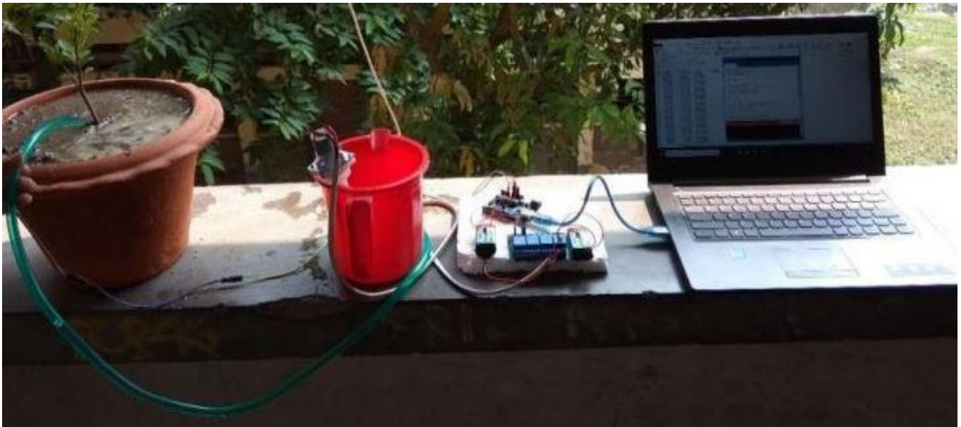
Fig 2. DEVICE SET UP FOR SMART IRRIGATION SYSTEM
