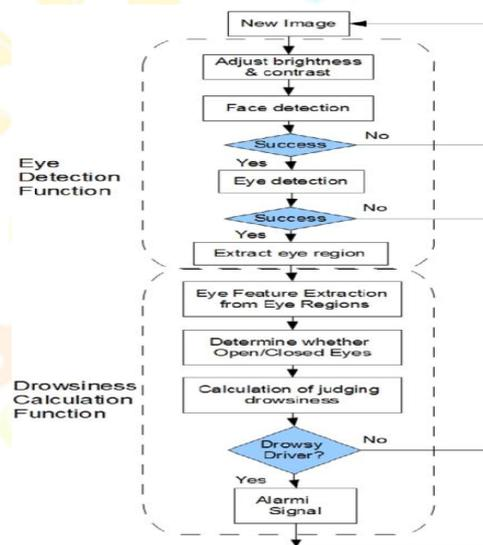
Figure 4.1: Flowchart for entire process of drowsiness detection system
