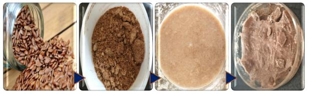
Fig 1.2 Extraction process for fenugreek seed gum
