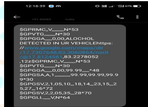
Figure 8: SMS for alocohol detected
