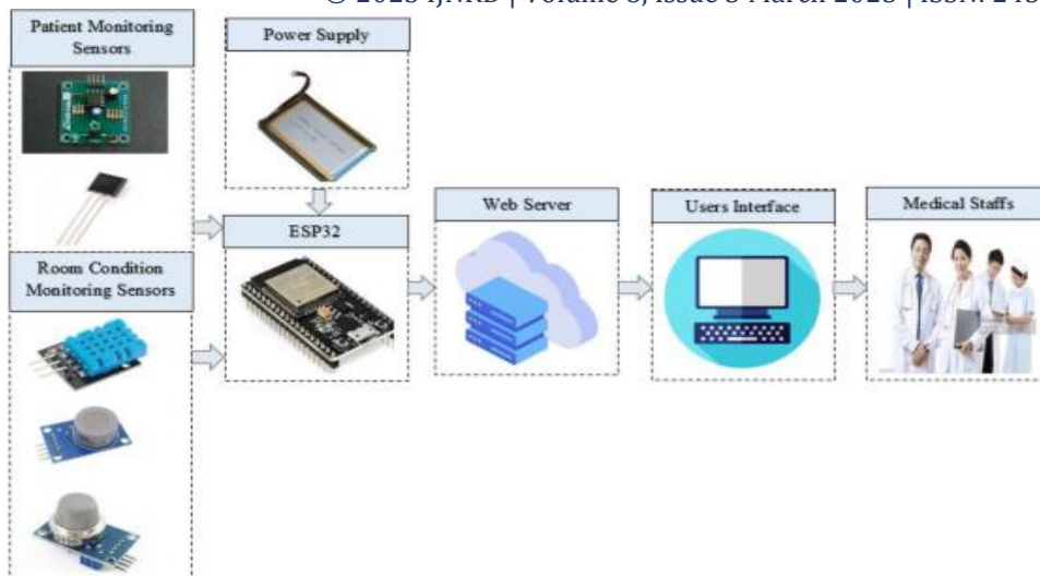
Fig a: The overall system architecture of the healthcare monitoring system
