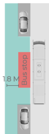
Fig ii - Bus stop clear width (Source-ITDP guidelines)
