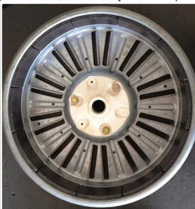
Fig. 4 Generator Stator (VWMM)
