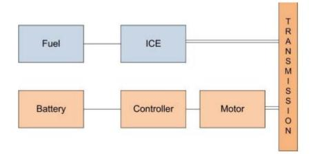
The two input of driving force makes the modelling of HEV and its components more complex than conventional vehicles. Mathematical modelling includes comprehensive, practical, updated, and easy to implement schemes.
