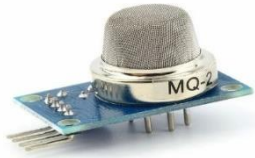
Fig 4. MQ2 Gas Sensor
