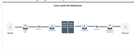
Fig. 7. Low level architecture of proposed chat application
