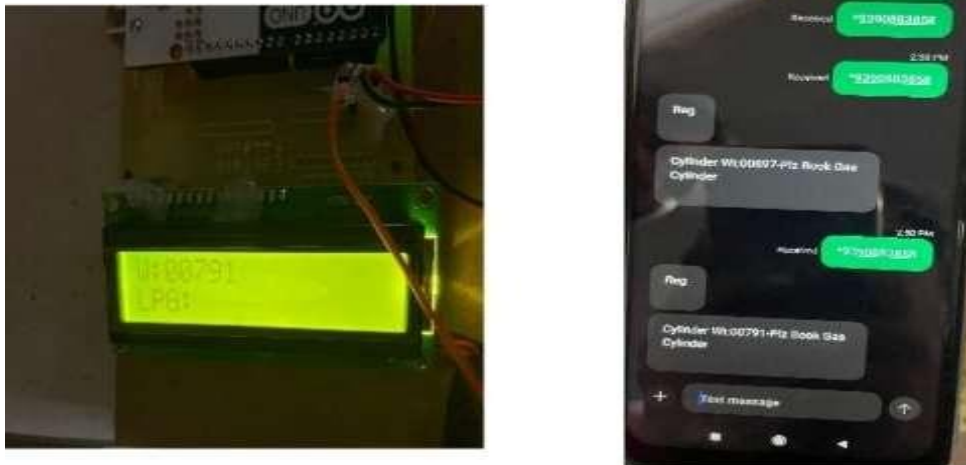
Fig. 6.3 LCD display when the gas level is below the threshold level
