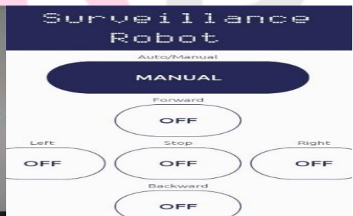
Fig 5.5:Manual mode is operated to move the robot, to detect the object, to start the Buzzer sound in Backward direction
