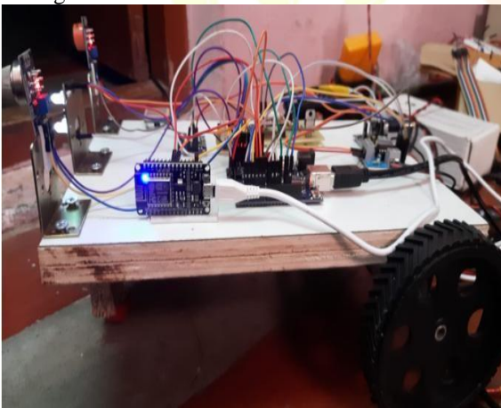
Figure 4.1 Working model of a smart in-vehicle alcohol detection and speed control system is designed
