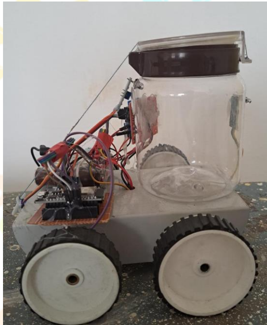
Fig 2: Automated dustbin with smart level detection
