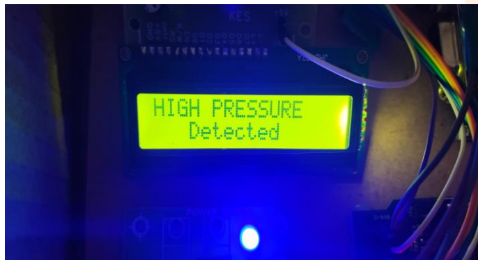
Fig 5.3: WHEN THE HIGH PRESSURE IS DETECTED THEN SMS SENT TO THE REGISTERED CONTACT
