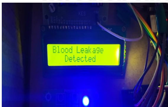
Fig 5.4: WHEN THE BLOOD LEAKAGE AND PRESSURE IS DETECTED THEN SMS SENT TO MOBILE
