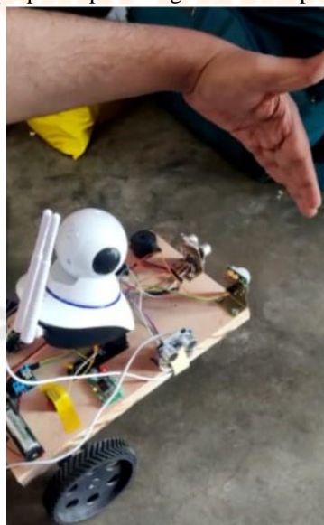
Fig:Proposed patrolling robotic vehicle,when intrusion detected
