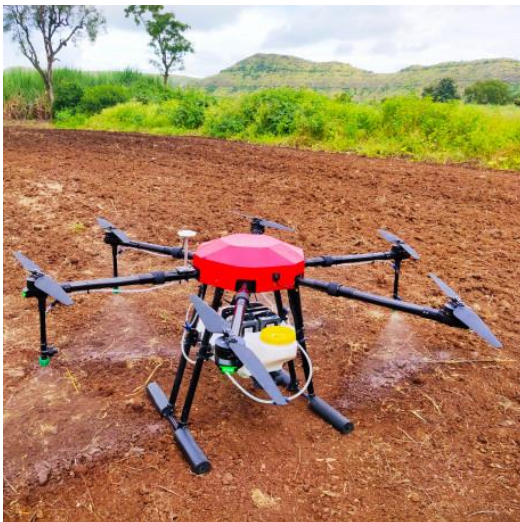
Fig 13. Drone for Spraying Pesticides
