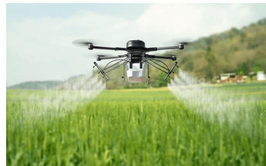
Fig 11 Drone for Spraying Pesticides.
