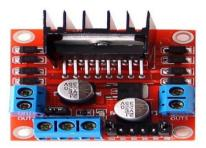
The motor driver is a key component in the automatic weed detection and cutting system, as it controls the movement of the cutting blade and other motors in the system. The motor driver is typically connected to the Raspberry Pi and receives commands from it to control the rotation, speed, and direction of the motors.
