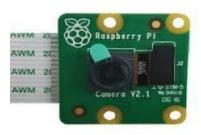
The camera module is an integral part of the automatic weed detection and cutting system, as it is responsible for capturing images of the crop field for weed detection. The camera module is typically connected to the Raspberry Pi, which processes the captured images using deep learning algorithms for weed detection
