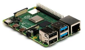
Raspberry Pi, a small-sized, single-board computer, plays a crucial role in the automatic weed detection and cutting system project. It serves as the central control unit that manages the system's overall functioning. Raspberry Pi offers several functionalities that are utilized in the project, including image processing, data analysis, decision-making, and motor control.
