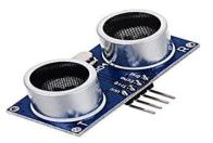
The ultrasonic sensor is a key component used in the automatic weed detection and cutting system for detecting the presence of weeds in the vicinity of the cutting blade. Ultrasonic sensors utilize sound waves at a frequency higher than the human audible range to measure distances and detect objects based on the time taken for the sound waves to reflect back.
