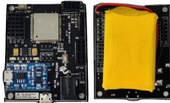
Fig 5: ESP 32 Strom Board
