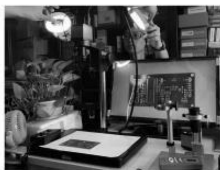
Fig 3.1 PCB image acquisition system consists of light source, workbench support, camera and image process unit
