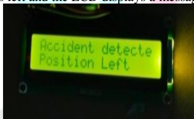
Fig5.6 Position indication during the accident condition of vehicle (Left)
