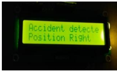
Fig5.8 Position indication during the accident condition of vehicle (Right)
