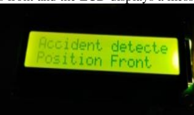
Fig5.7 Position indication during the accident condition of vehicle (Front)
