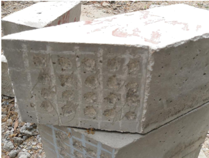
fig: 3.5.2 Specimen that had chipped at regular intervals after 28 days of curing at 45^{\circ}
