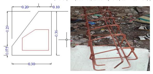
Fig No. 4 Design Copper beam.
