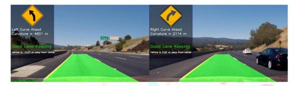
As we can see the curved lanes are being perfectly detected as well as the distance from the centre is also corrected mentioned in the output.
