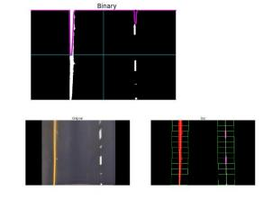
Here, the red and pink color represents the 'hot' pixels for the left and right lane lines respectively. Furthermore, the line in green is the polyfit for the corresponding 'hot' pixels.
