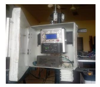
Figure 5: Assembling of Constructed Air Pollutant Data Logger unit for data storage for Laboratory Test
