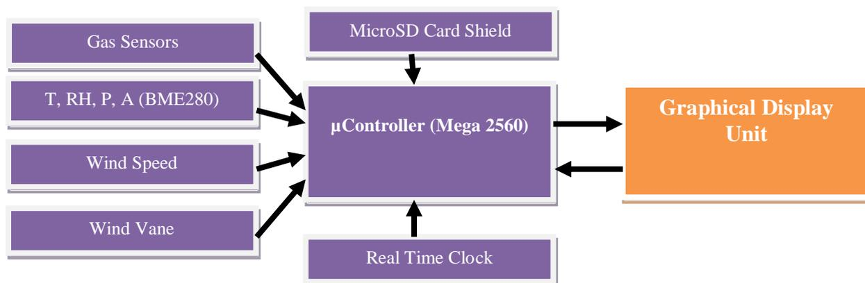
Figure1. The Block Diagram of Gas and Dust Monitoring Device
