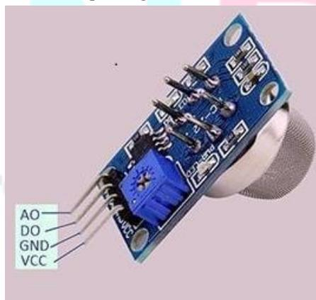
Figure 2. Picture View of Sample of Gas Sensor
