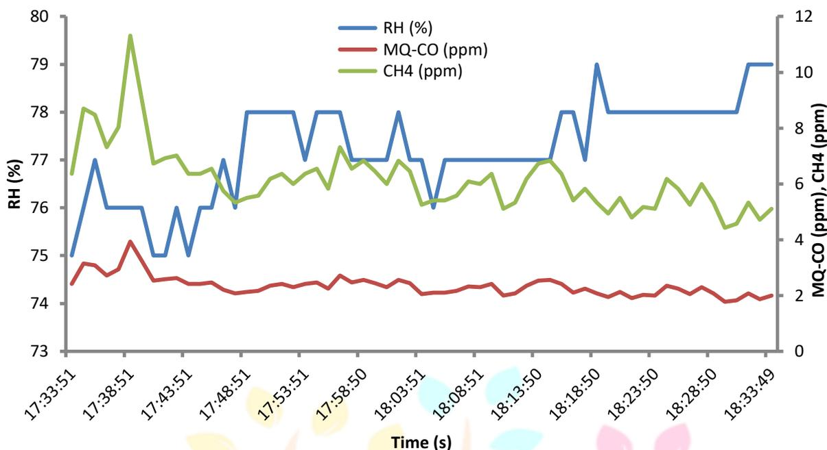
Figure 8. Sample Data Analysis at Igbatoro, Akure, Nigeria (RH and Gas Release from Dump Site) on 1/3/2023.
