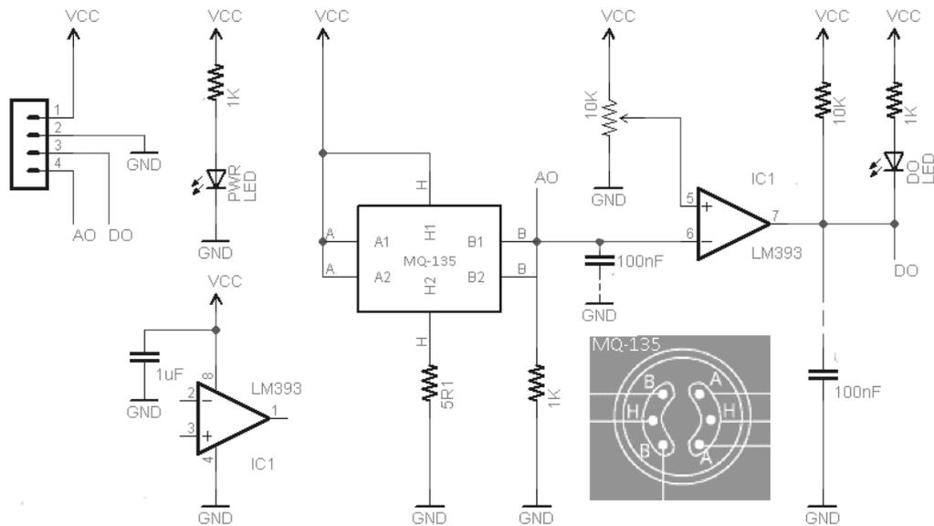
Figure 3. Digital Output Circuit for Gas Sensor Output
