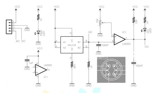
Figure 3. Digital Output Circuit for Gas Sensor Output
