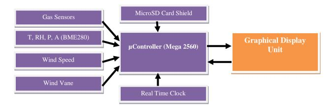
Figure1. The Block Diagram of Gas and Dust Monitoring Device
