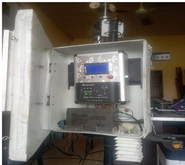
Figure 5: Assembling of Constructed Air Pollutant Data Logger unit for data storage for Laboratory Test
