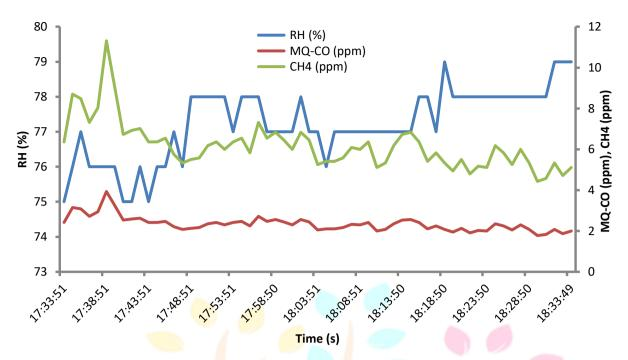
Figure 8. Sample Data Analysis at Igbatoro, Akure, Nigeria (RH and Gas Release from Dump Site) on 1/3/2023.
