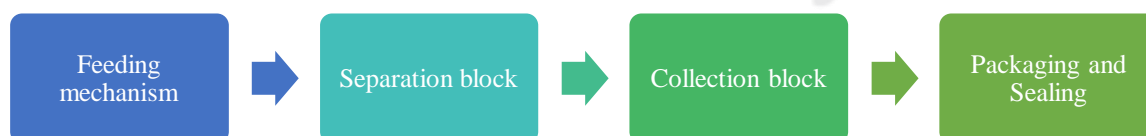
Figure 1: Represent the block diagram of green leaf separating machine.
