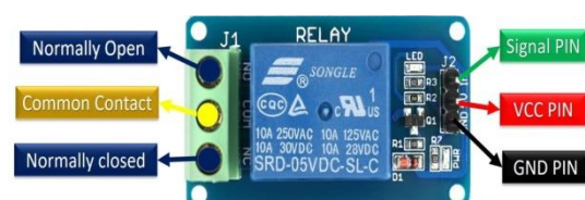
Fig 4.5 5V Relay Module Pin Configuration
