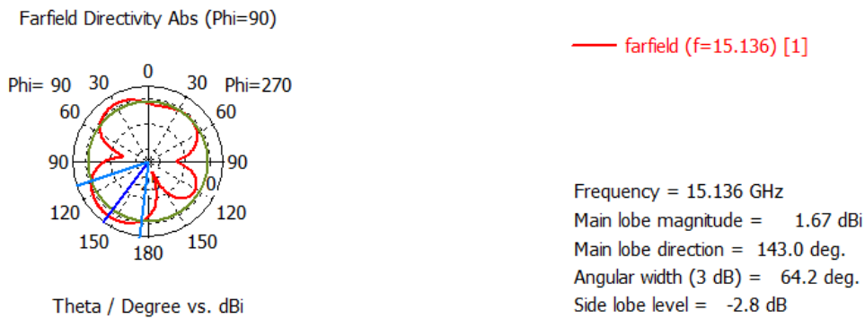
Fig. 6. Polar plot at 15.136 GHz
