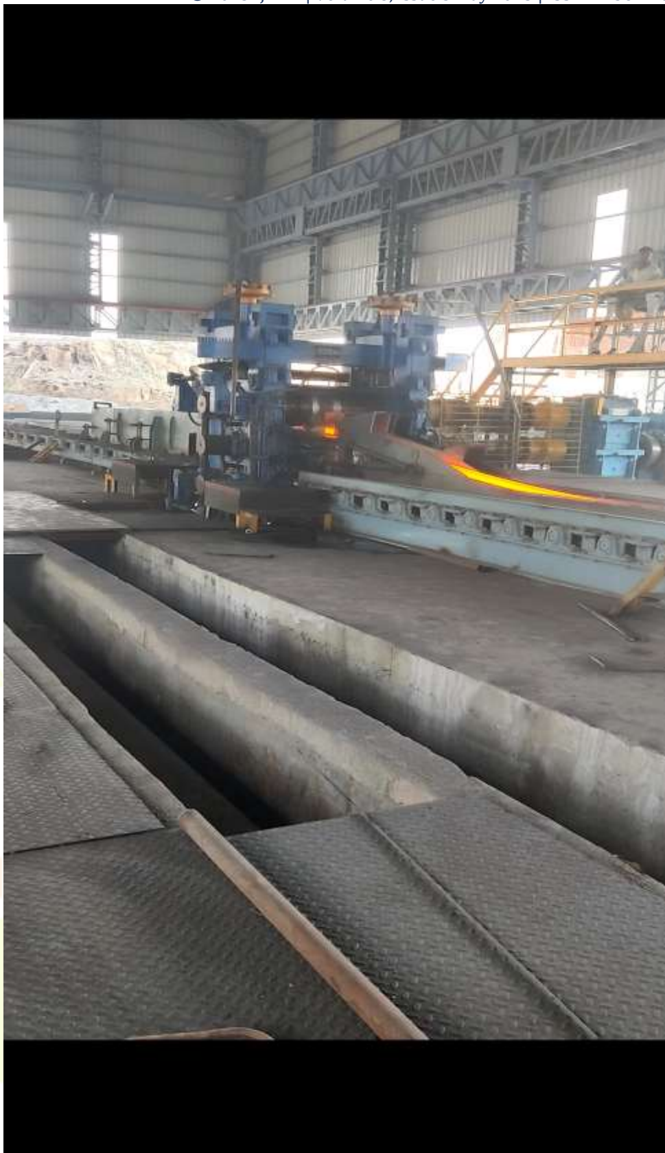
Figure 1.12 Rolling Mill Hot Iron Bar Rolled front and Back For TMT
