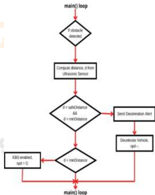
Fig. 7. Flow diagram for EBS algorithm
