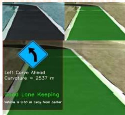
Fig. 12. V-Assist model captures the frame and processes the image to identify left turn
