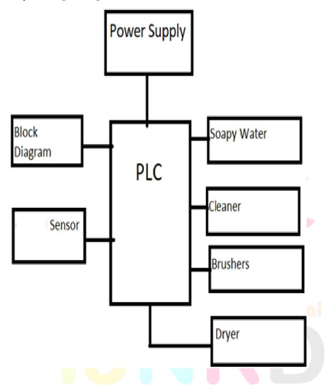
Fig. Block Diagram of car washing system using PLC
