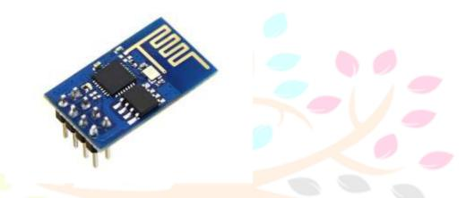
The ESP-01 has 8 pins, including 2 GPIO pins. - Antenna on a PCB trace. (As in the figure above) The ESP-02 has 8 pins, including 3 GPIO pins. –U-FL antenna connection. Seven of the ESP-03's 14 pins are GPIO pins. antenna made of ceramic.
