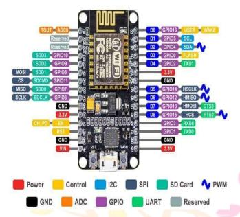
The Node MCU (Node Micro Controller Unit) is an open-source software and hardware development environment built around an inexpensive System-on-a-Chip (SoC) called the ESP8266. The ESP8266, designed and manufactured by Espress if Systems, contains the crucial elements of a computer: CPU, RAM, networking (Wi-Fi), and even a modern operating system and SDK. That makes it an excellent choice for Internet of Things (IoT) projects of all kinds.
