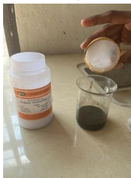
fig.3: neutralizing the acid solution by adding the desired amount of sodium hydroxide
