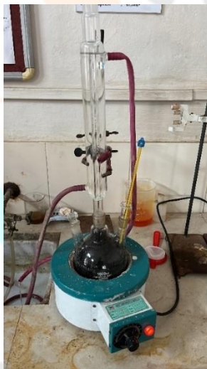
fig.2: experimental setup for the hydrolysis process
