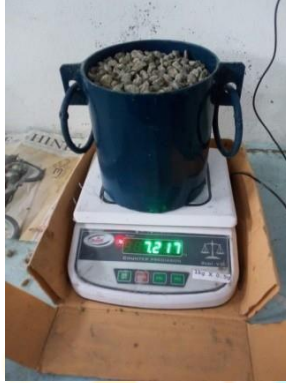
FIG. 5.5 BULK DENSITY OF COARSE AGGREGATE
